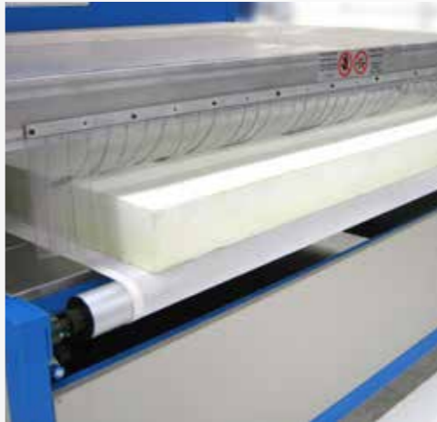
> RF drying of mattresses 400 kg/h throughput
