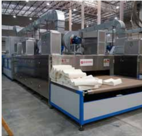
> RF drying of pillows 300 kg/h throughput
