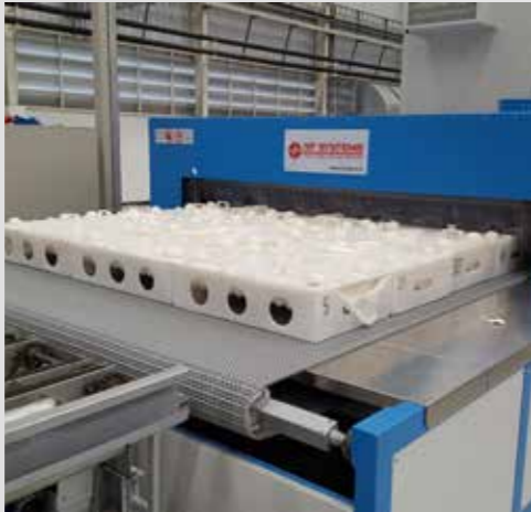
> RF vulcanization of pillows Vulcanization in plastic molds
